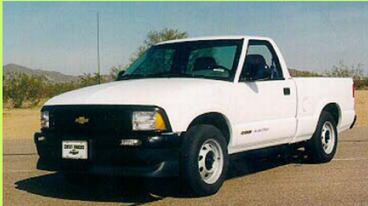
Chevrolet S10 EV: 95 mile range, 9 hour charge time with NiMH batteries
