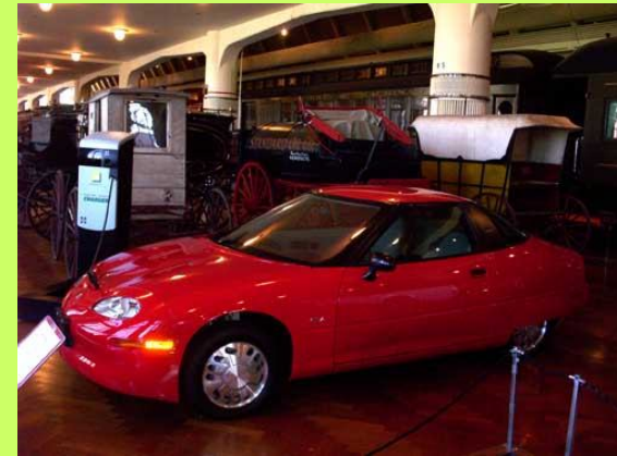
General Motors EV1: 140 mile range, 7 hour charge time with NiMH batteries
