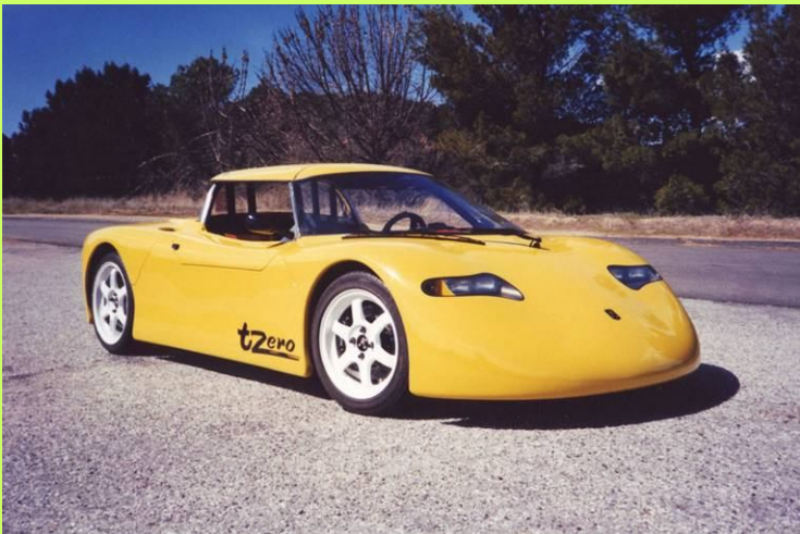
AC Propulsion tZero: 302+ mile range, 3.5 hour charge time with Lithium Ion batteries
