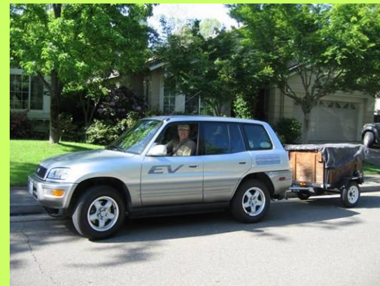
Toyota RAV4 EV: 94 mile range, 5 hour charge time (2002 model) with NiMH batteries
